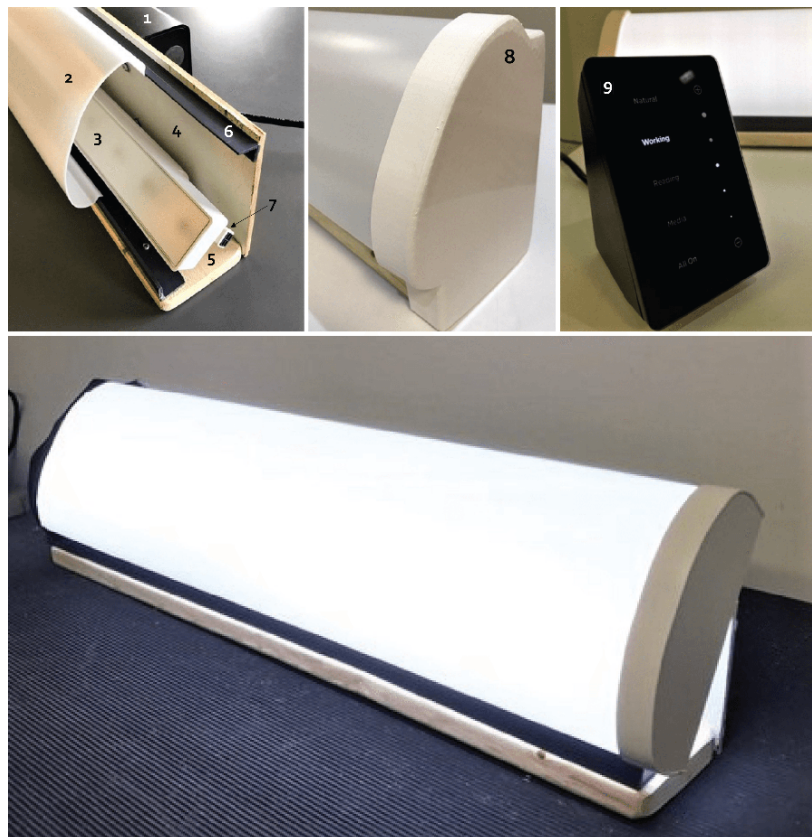
Figure 3. Components of the desktop luminaire that was custom-built by the LRC for use in this study (top): (1) satellite link controller, (2) light diffuser, (3) LED linear accent, (4) plywood housing back, (5) pine board base, (6) ½-in. × 1-in., PVC 90° angle (×2), (7) connector cable, (8) installed endcap, (9) touchpad interface. A prototype of the assembled device is shown in operation below.
